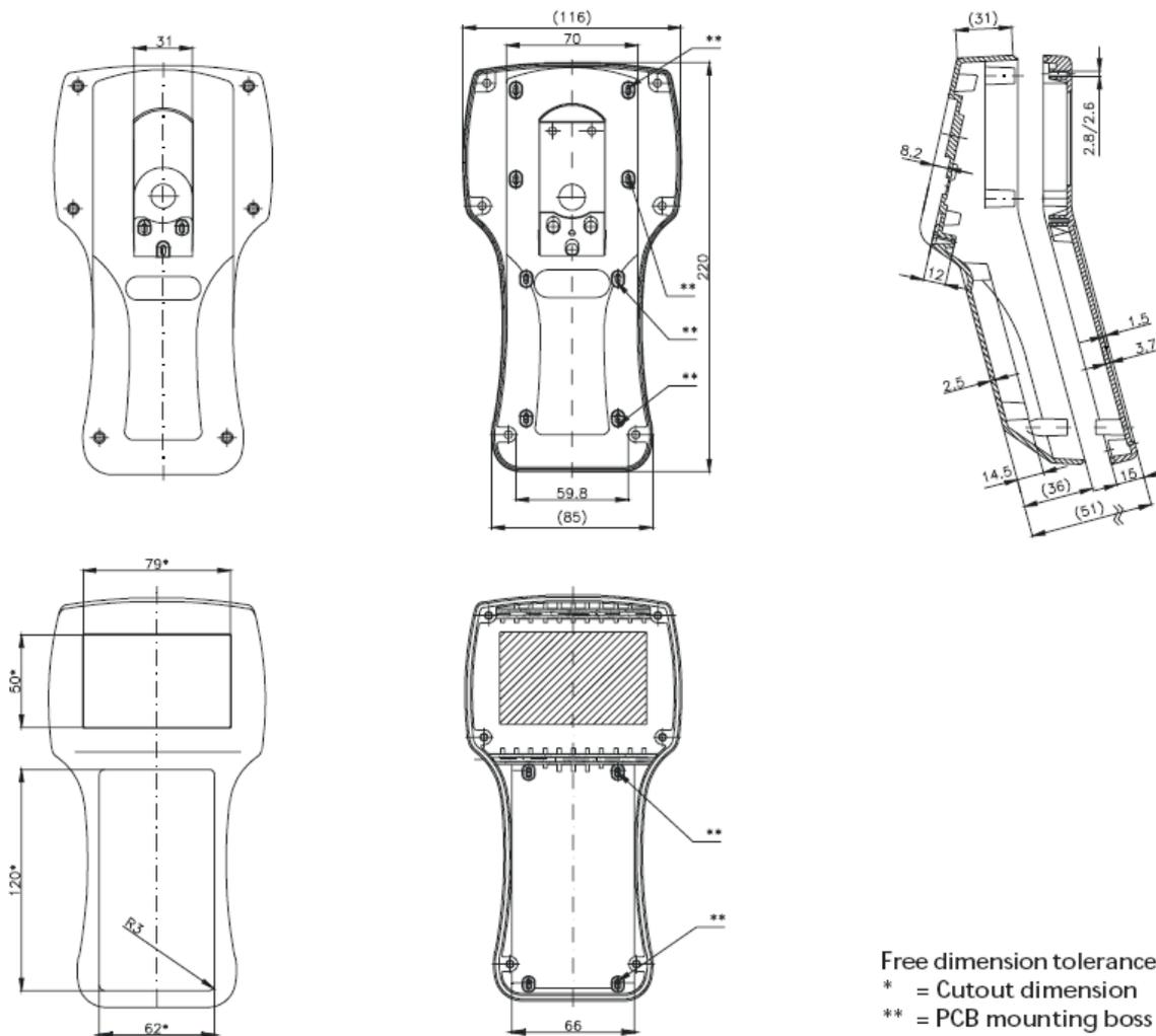
Free dimension tolerance to DIN 16901-130
