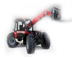
Tractors Telehandler In the Security System Anti Rollover ARMS monitors during operation of the machine working angles. In the case of approaching the corner of safety, the operator is alerted by an acoustic signal of view. At the overcoming of the angles of safety, the vehicle is stopped or brought within the limits of the security parameters.
